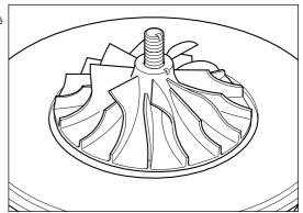
Brush the thread and nut face with an anti-seize compound to avoid loss of alignment during torque tightening.
