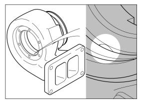
To replace turbine housing apply anti seize compound to bearing housing locating bore of the turbine housing.
