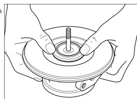
Gently tap the oil seal plate (43) with a soft hammer to seat in position.
