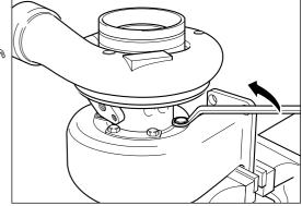
Using a soft hammer, tap turbine housing down against soft bench surface. As bearing housing and compressor housing assembly comes loose gently lift it out of turbine housing engagement
