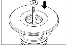
Using clean engine oil, lubricate the thrust bearing (12). Install the thrust bearing.
