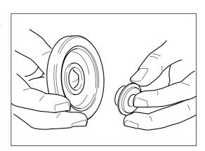
Using piston ring expander pliers remove and discard split ring seal, compressor (16) \* from oil slinger.
