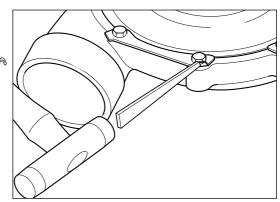
Ensure rotor assembly freely rotates.
