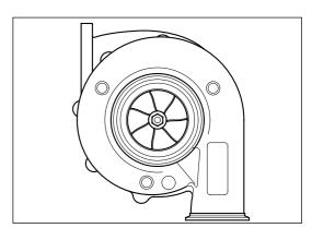
Where practical, check for cracked, bent or damaged turbine wheel blades.
