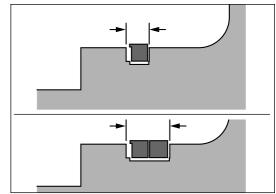
Inspect split ring seal, turbine (13)\* groove walls for wear. If groove width exceeds recommended maximum replace assembly.
