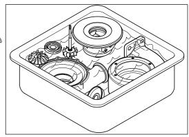
Dry the components using compressed air.
