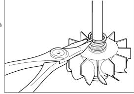
With bearing housing (4) on a flat clean surface, use suitable circlip pliers to remove insert, retaining ring (66).
