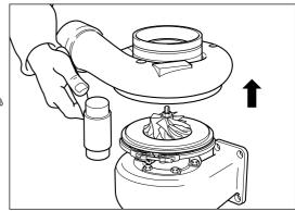
The bearing housing to compressor housing joint is fitted with o-ring seal, compressor (41). This seal should be removed and discarded at this stage.
