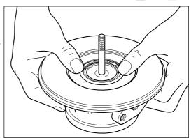
Use soft hammer and drift to ensure retaining ring (66) is properly located.
