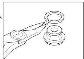
Install the oil baffle (33).
