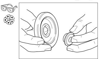
Transfer assembly from fixture locating on turbine wheel nose to one locating on bearing housing.
