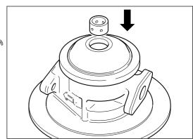
Fit the outer retaining ring (64)  $\star$  with the bevelled edge facing the bearing.
