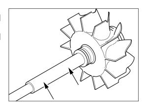
Inspect the bearing journals for excessive scratches and wear. Where scratching is excessive or where either journal diameter is less than the recommended minimum of 12.19 mm (0.48 in) replace the assembly.
