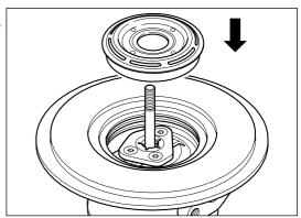
Apply a small amount of engine oil to the o-ring and insert the o-ring seal, bearing housing (32) \*.
