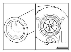
Always refer to *Cleaning of Housings* to clean housing. Rotor components can be cleaned using a non metallic bristle brush.
