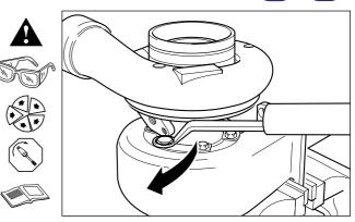
Ensure rotor assembly freely rotates.
