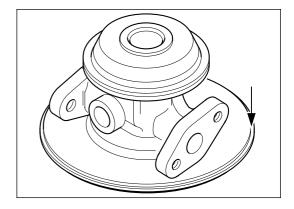
Check retaining ring (66) retaining ring groove does not exceed a maximum width dimension of: 2 mm (0.079 in).
