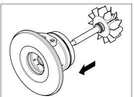
Support the assembly turbine wheel (6) in a suitable fixture.
