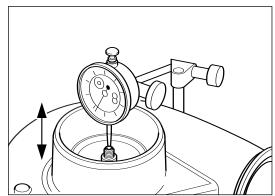
Check the radial movement at compressor impeller nose using a dial gauge.
