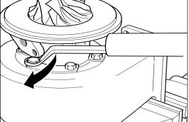
Check thrust clearance using a dial gauge. Ensure clearance is within MIN/MAX values shown in Service Data Sheet
