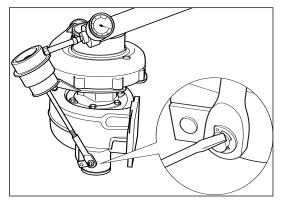
Ensure rotor assembly freely rotates.
