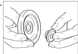
Transfer assembly from fixture locating on turbine wheel nose to one locating on bearing housing.
