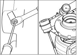
With actuator end link disassembled from valve mechanism, apply air pressure (Max 3 bar, 45 lbf/in2) and check for actuator movement.
