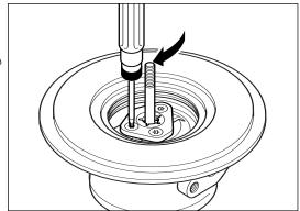
Install new split ring seal, compressor (13) \* to oil slinger (31).
