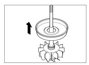
Carefully remove the split ring seal / seals, turbine (13) \* and discard.
