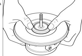
Gently tap the oil seal plate (43) with a soft hammer to seat in position.
