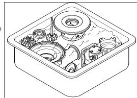
Dry the components using compressed air.
