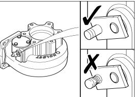
The same failure conditions can also lead to elongation of the rod end bore which locates on the lever arm pin. This must not exceed 0.50 mm (0.020 in).
