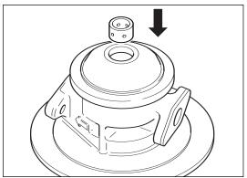
Fit the outer retaining ring (64)  $\star$  with the bevelled edge facing the bearing.
