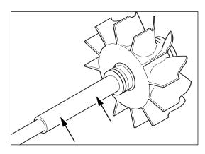
Inspect for cracked, bent or damaged blades.
