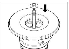
Using clean engine oil, lubricate the thrust bearing (12). Install the thrust bearing.
