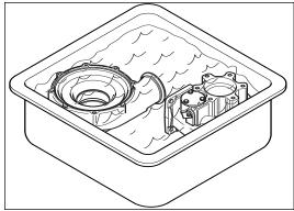
Dry the components using compressed air.
