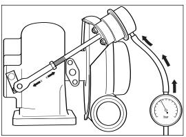
If there is no movement, replace actuator in accordance with Actuator Removal and Actuator Replacement.
