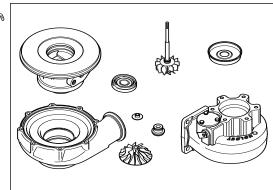
Soak the components in a non-corrosive low flash point metal cleaner to loosen deposits.
