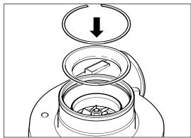
Hold one end of the retaining ring in position in its compressor cover groove. Press the remainder of the retaining ring into position using free hand.
