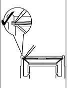
Secure turbine housing flange in vice. To refit compressor housing, lubricate new o-ring seal (41) with clean engine oil and install into retaining groove.
