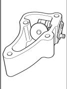
Torque tighten setscrews to value specified in **Service Data Sheet** ensuring that lockplates and washers are refitted.
