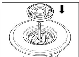
Apply a small amount of engine oil to the o-ring and insert the o-ring seal, bearing housing (32) \*.
