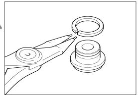
Install the oil baffle (33).
