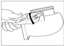
Radial cracks can occur around the valve seat when the turbocharger has been abused or overheated. It is possible to inspect for cracks using a torch. Check that rivet attaching valve to linkage is not loose.
