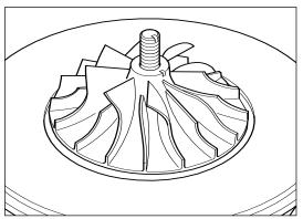
Brush the thread and nut face with an anti-seize compound to avoid loss of alignment during torque tightening.
