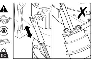
Inspect wastegate bracket for cracks at the actuator fastener locations.
