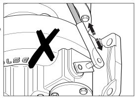
If there is movement, check valve mechanism for seizure in accordance with Wastegate Mechanism Check.
