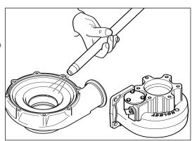
Scale like deposits, if any, must be removed by using a non metallic bristle brush. After removing the deposits, re-wash and dry the components.
