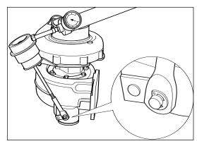
Ensure rotor assembly freely rotates.
