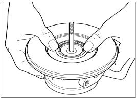
Use soft hammer and drift to ensure retaining ring (66) is properly located.
