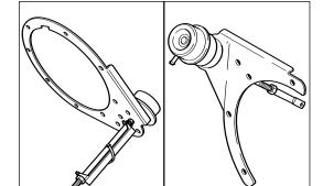
Thread new end-link several turns on to the shaft of the new pre-set actuator assembly.
