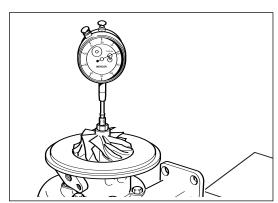
Check compressor end radial movement using a dial gauge. Ensure clearance lies within MIN/MAX TIR (Total Indicator Reading) values shown in Service Data Sheet
