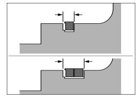
Inspect the bearing journals for excessive scratches and wear. Where scratching is excessive or where either journal diameter is less than the recommended minimum of 12.19 mm (0.48 in) replace the assembly.
